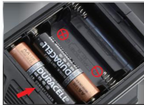
Put in 4 AA battery, close the cover ,notice correct polarity
