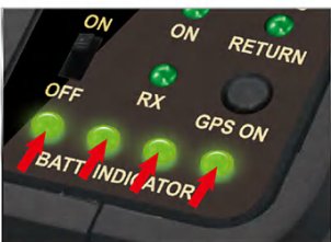
When transmitter and RC boat are both power on, the four green lights on the transmitter turn on.
