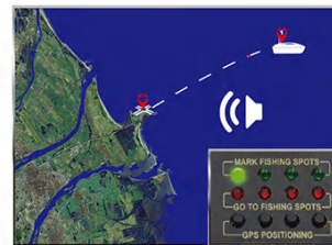
When the boat arrive at the spot by GPS autopilot, Boat stop, the red light will be off and transmitter will make beep sound to indicate boat has arrived to the marked fishing spot.
