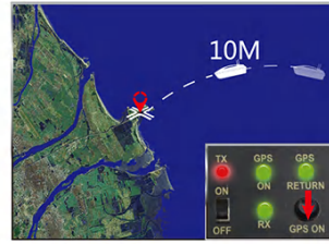
After the boat driven to some distance, Press button GPS ON over 1 second, GPS RETURN green light is solid on, the boat will return back to the original point automatically. When arrive at original point, you will hear a beep sound on TX, GPS RETURN light will be off.
