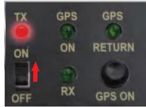
Switch on power, TX LED light on. Note: Switch on Transmitter firstly before connect power battery with boat.
