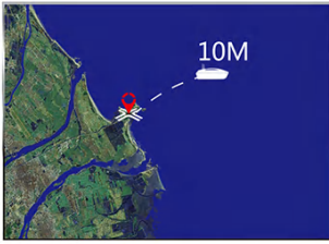
Control the boat to a spot 10 meters away from the shore. This location to be the original point that you need to set up.
