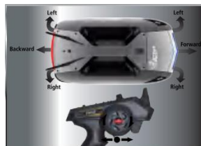
Pull the trigger back, the boat moves forward; push the trigger forward, the boat moves backward; rotate the wheel anti-clockwise, the boat turns left; rotate the wheel clockwise, the boat turns right.
