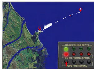
If you want boat gets back to the marked fishing spot, Press GPS POSITIONING button over 1 second, relevant red light will be solid on, boat go to marked fishing spot by GPS autopilot.
