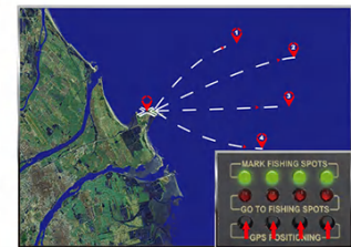
You can set up 4 different fishing spots by pressing the corresponding GPS POSITIONING button over 5 seconds.
