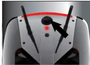
Switch on power button on rear top of the Boat handle, Power light turns on. If not use boat for short time, switch off Power button. If not use boat for long time, You must disconnect battery with boat.
